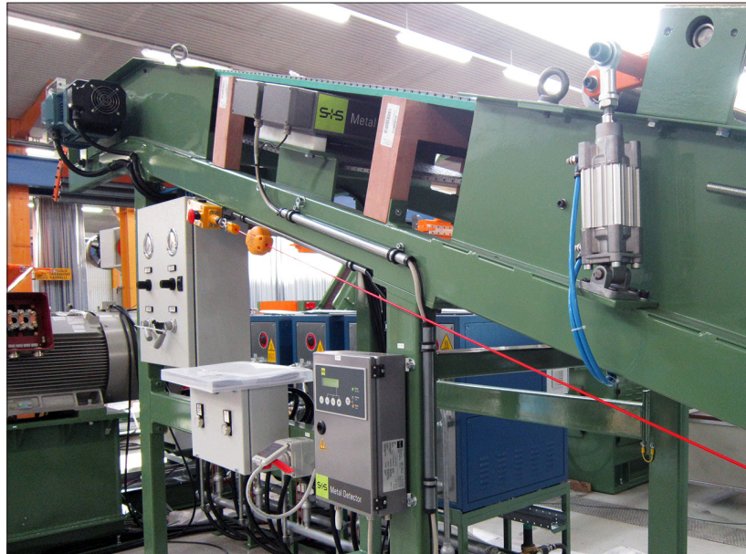
Plate-type metal detector of type ELS installed below the feed conveyor belt of a Marangoni Meccanica S.p.A production line.
